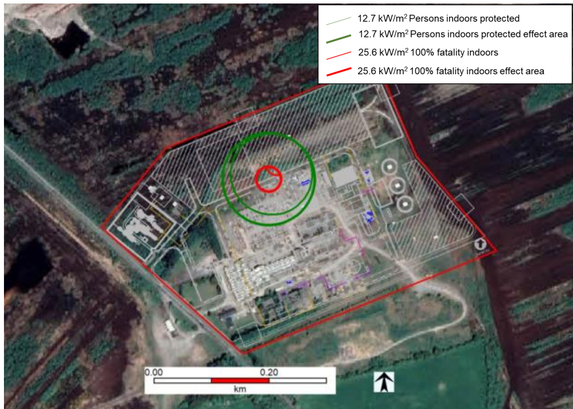
Figure 11 Natural Gas Pipeline Release and Jet Fire: Indoor Fatality Thermal Radiation Contours
