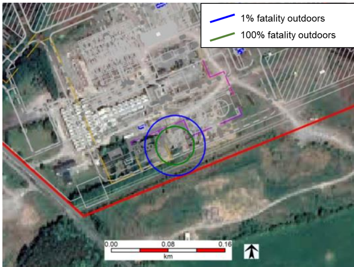
Figure 28 LPG Tank Rupture and Fireball: Outdoor Lethality Contours
