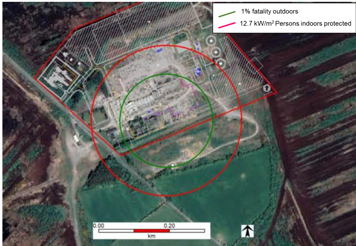
Figure 35 LPG Tanker Rupture and Fireball: Outdoor Lethality Contours
