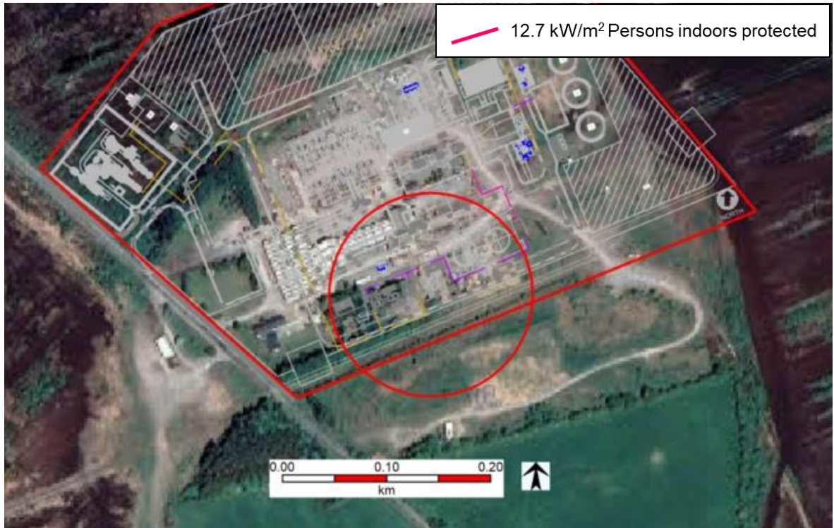
Figure 29 LPG Tank Rupture and Fireball: Indoor Lethality Contours
