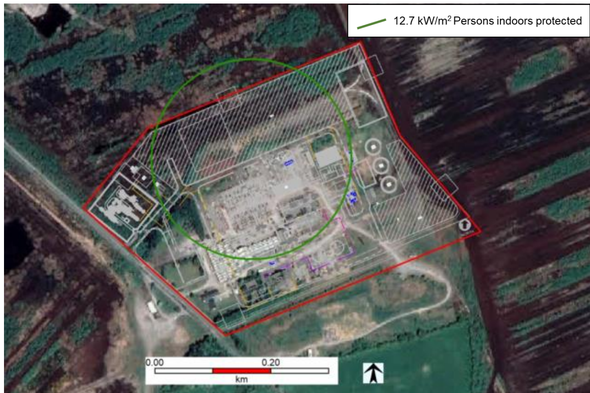
Figure 17 Natural Gas Pipeline Rupture and Fireball: Indoor Fatality Contours
