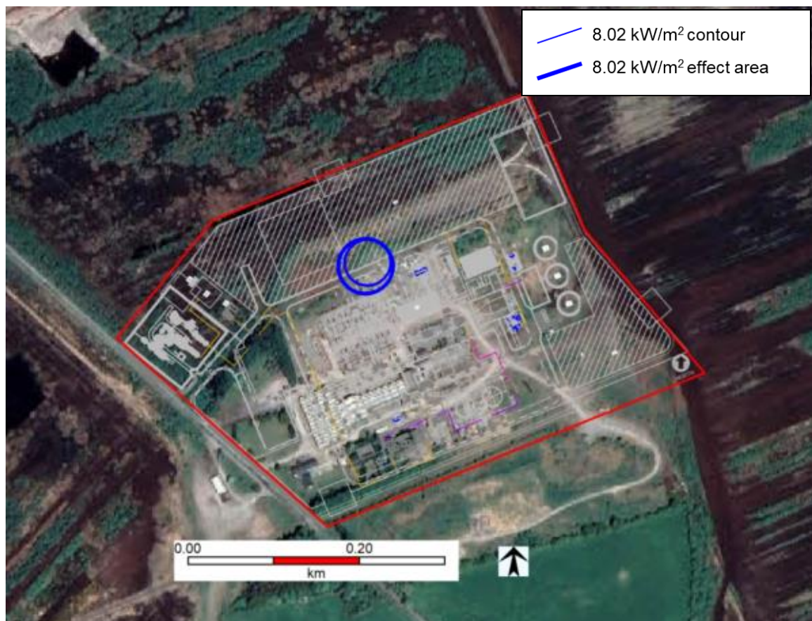
Figure 12 Natural Gas Pipeline Leak and Jet Fire: Thermal Radiation Contours Corresponding to 1% Fatality Outdoors
