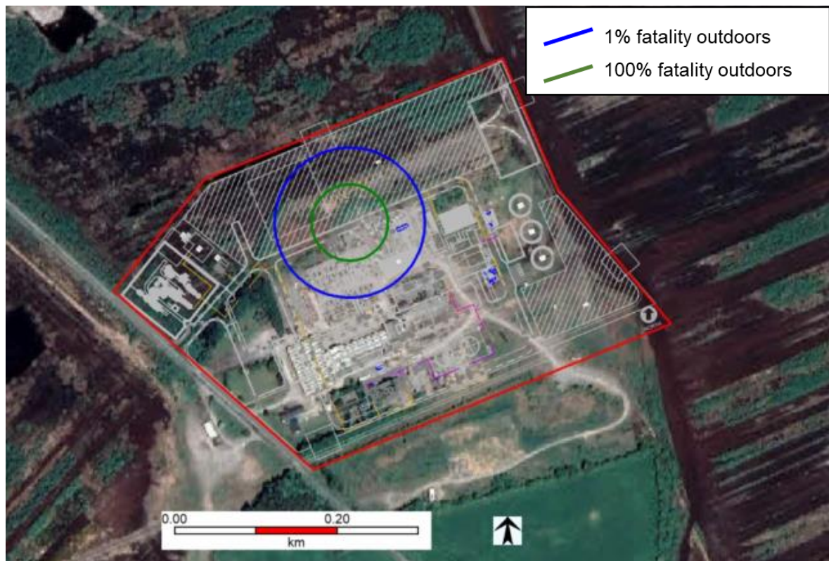
Figure 16 Natural Gas Pipeline Rupture and Fireball: Outdoor Fatality Contours
