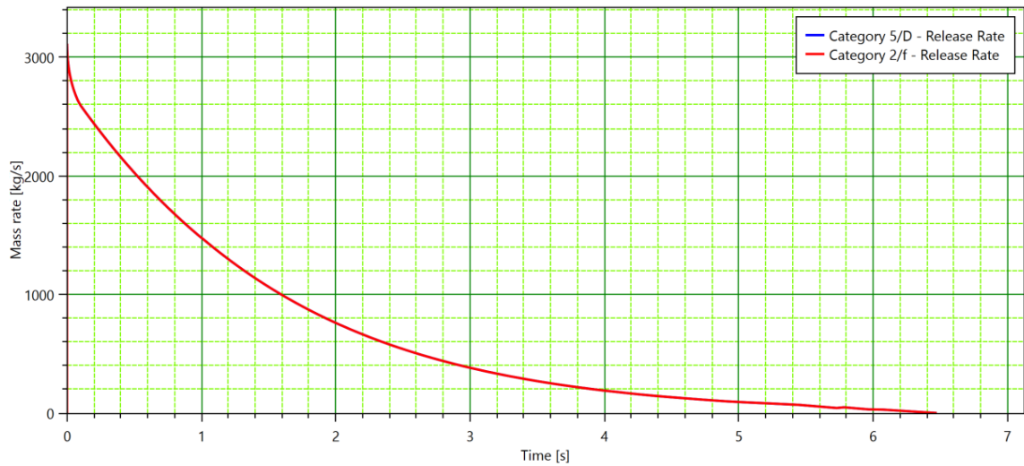
Figure 5 Natural Gas Pipeline Full Rupture: Release Rate vs Time
