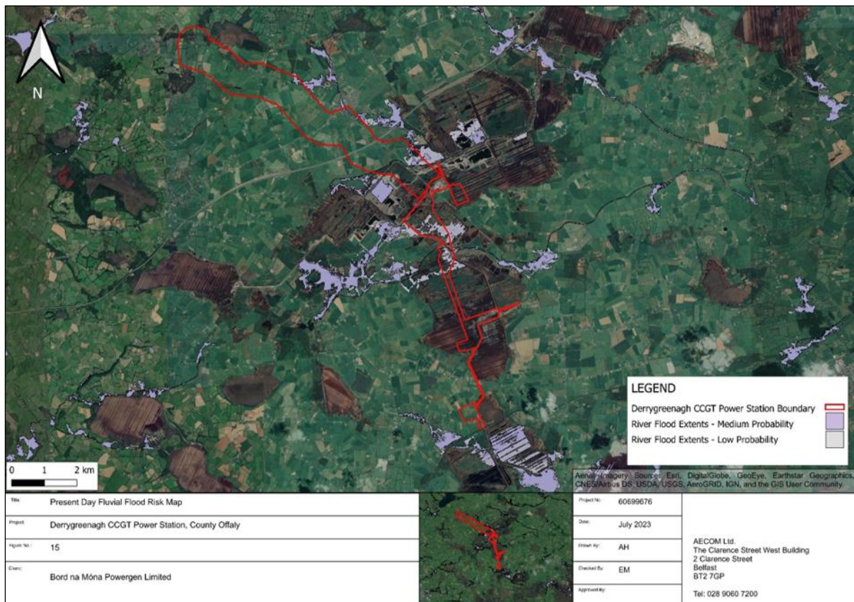
Figure 3.8: Present Day Fluvial Flood Extents: Proposed Development and Overall Project Area
