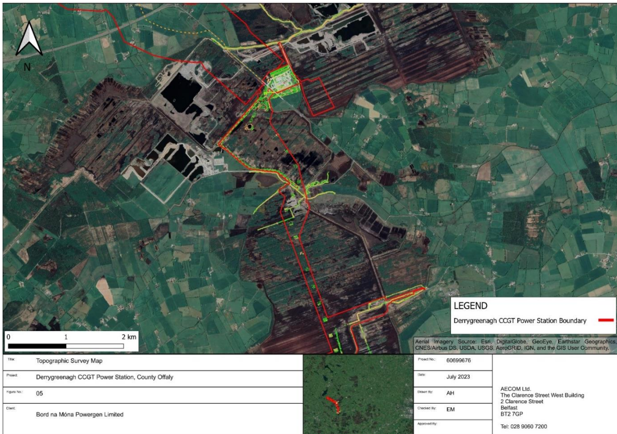
Figure 2.4: Topographic Survey: Power Plant Area, 220 kV Substation, process water discharge pipe and section of OHL
