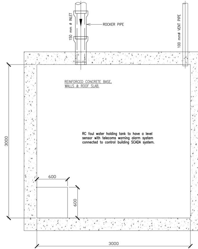
TYPICAL FOUL WATER HOLDING TANK SCALE 1:20
