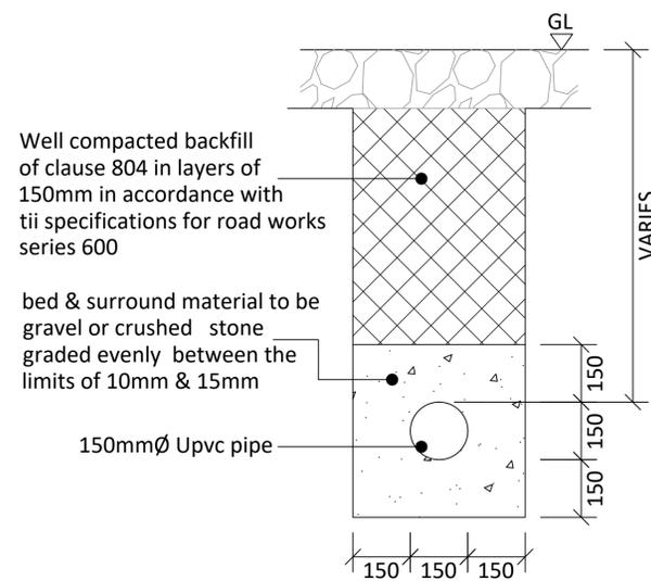
TYPICAL SECTION THROUGH FOUL/SURFACE WATER SEWER SCALE 1:10
